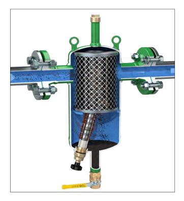
To purge the debris, the flexible magnetic stack is removed from the brass dry-well and, even while the system is still running, the drain valve is opened. Aided by the system pressure, the dirt and magnetite flushes out quickly and effectively. DIRTMAG<sup>®</sup> magnetic dirt separators accomplish 21/2 times the ferrous impurities removal performance of standard dirt separators, delivering up to 100% elimination efficiency.
