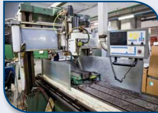
PRO Engineer Software station for MOULD design connected with a 4 AXIS CNC mill with a long up to 3 meters table for big Moulds production.
